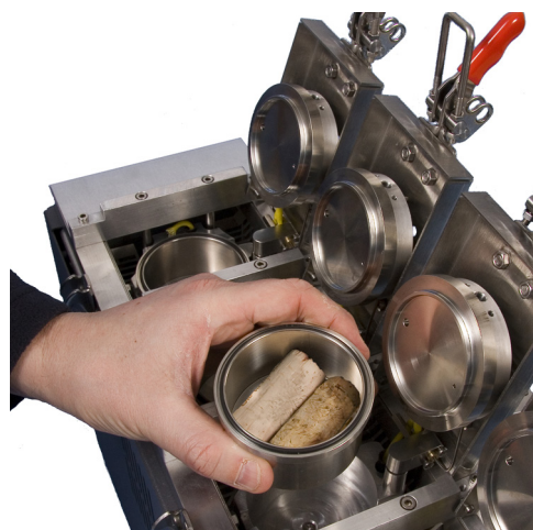
Figure 1: The Micro-Chamber/Thermal Extractor, showing samples being placed in the instrument ready for sampling.
