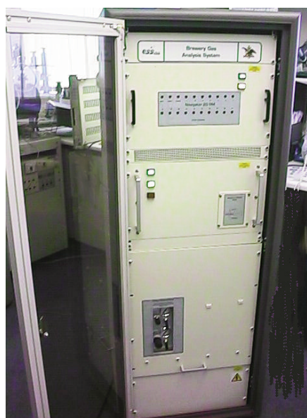
Figure 7: A 19" rack-mounted TD-MS system.
